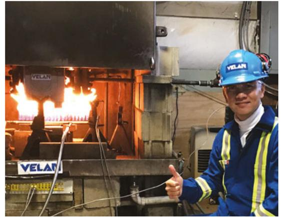
Duke Tran, Executive Vice-President, General Manager, Severe Service, at an independent lab witnessing the fire testing of five Velan valves including metal-seated ball valves and a Torqseal® 2.0 triple offset valve. Velan's very stringent testing requirements resulted in a 100% pass rate.
