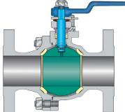
**Spilt-body ball valves SB-150/300/600** ASME 150, 300, 600 Full port: NPS ½–24 (DN 15–600) Regular port: NPS 2–24 (DN 50–600) Live-loaded, flanged
