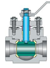
Top-entry ball valves TE-150/300/600 ASME 150, 300, 600 1480 WOG Full port: NPS <sup>3</sup>/8-6 (DN 10-150) Regular port: NPS <sup>1</sup>⁄2-6 (DN 15-150) Live-loaded, double packed, bellows seal, threaded, socket weld, butt-weld or flanged
