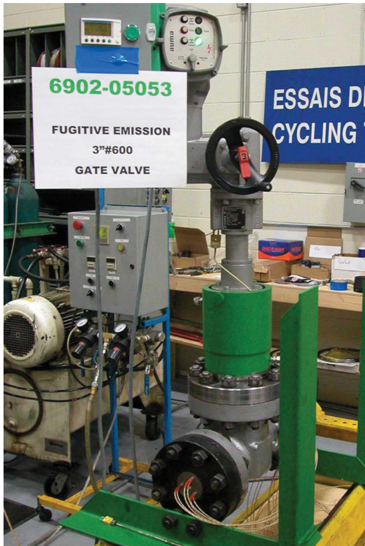
Fugitive-emissions R&D testing setup on a Velan 3" (80 mm) Class 600 gate valve, as part of Velan's ISO-15848-1 qualification program.
