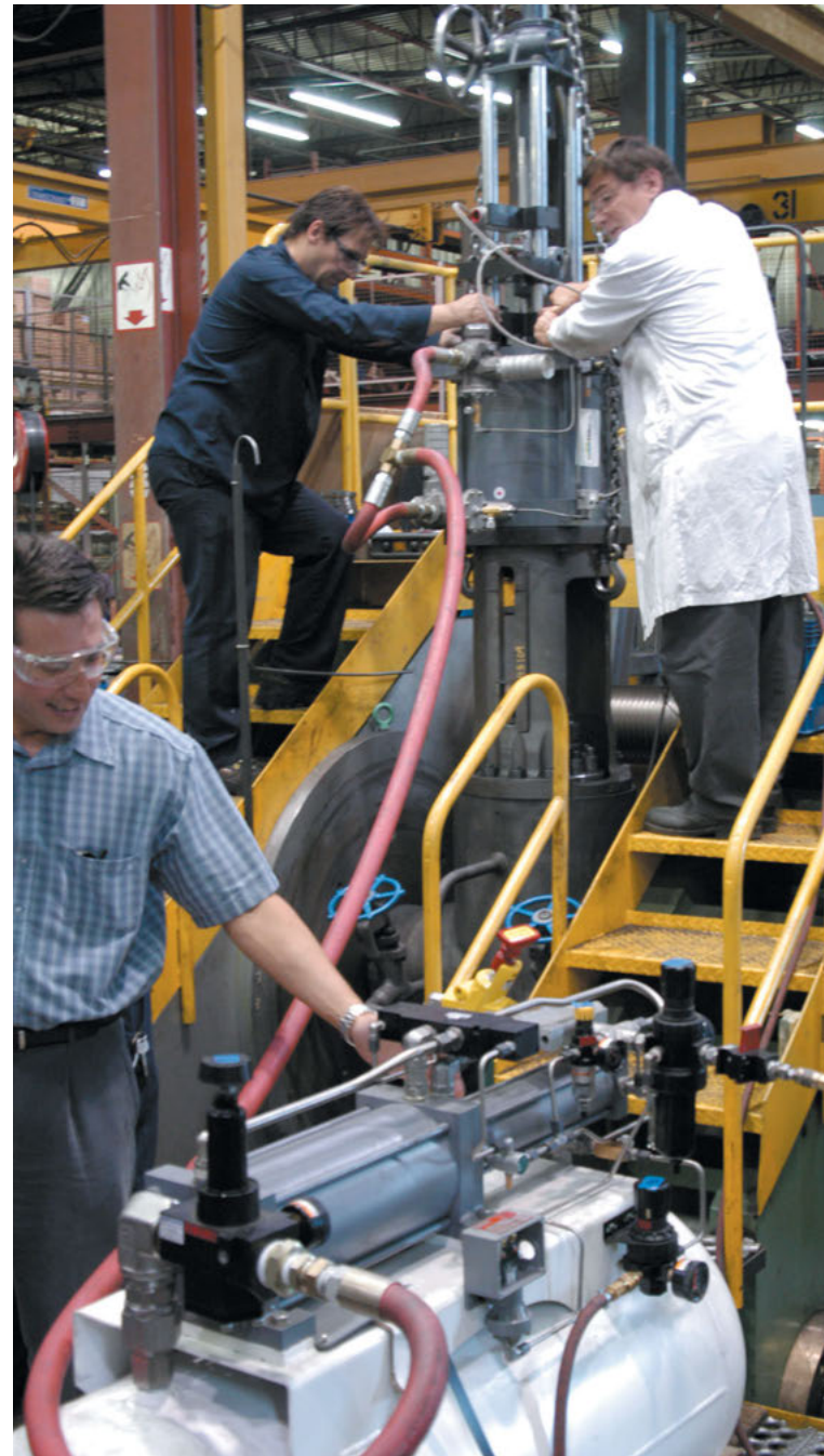
Fugitive-emissions R&D testing setup on a Velan 3" (80 mm) Class 600 gate valve, as part of Velan's ISO-15848-1 qualification program.
