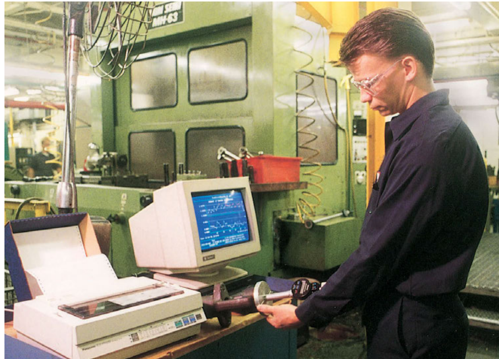
On-line statistical process control (SPC) is used on a y-pattern globe body after machining.
