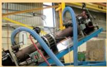
During testing, wafer check valves were cycled both vertically and, as seen here, horizontally.
