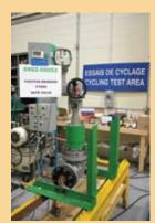
Cycle testing for fugitive emissions today targets 600, 900, and 1500 dass valves.
